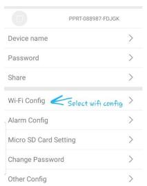
After selecting Wi-Fi Config, we are taken to a page where you can choose a network for the unit to connect to, and then type in the password for that wi-fi network. Press 'Confirm' when done to pair the unit with the router. You should see something that says "Set Success".
